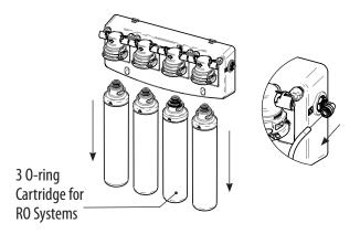
2 Disconnect all 4 cartridges and replace them with the blank cartridges included in this kit. Disconnect the inlet line from the system and drain excess water into a pail.
