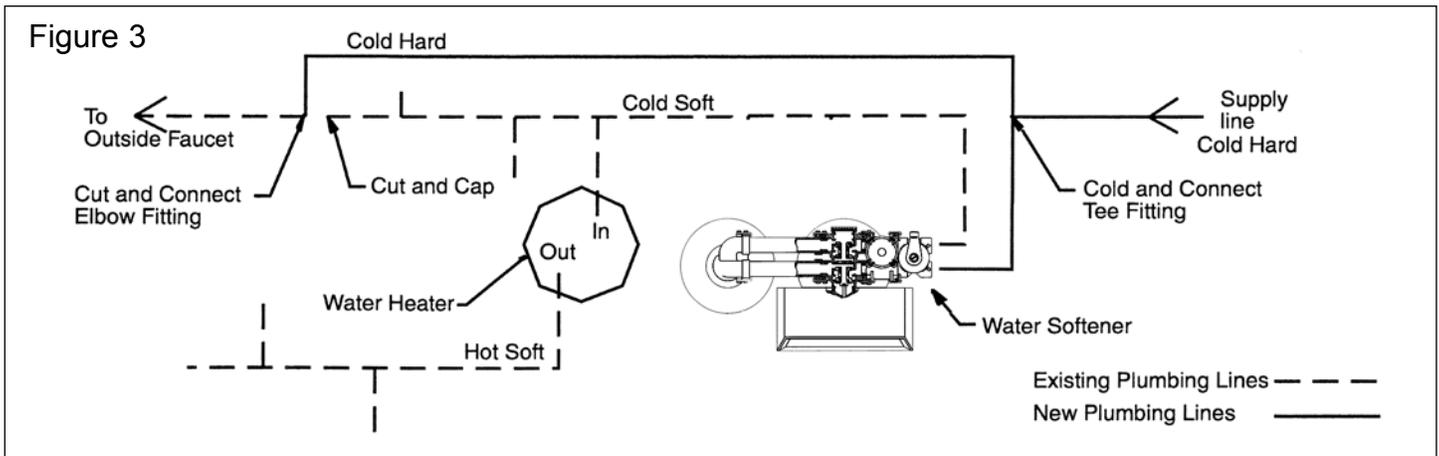
4. Attach the bypass valve to the control valve. Connect the inlet and outlet of the water softener to the plumbing in the house. The control valve must not be submitted to temperatures above 43°C (110°F). When sweat fittings are used, to avoid damaging the control valve, solder the threaded copper adapters to the copper pipe and then, using Teflon tape, screw the assembly into the bypass valve.
