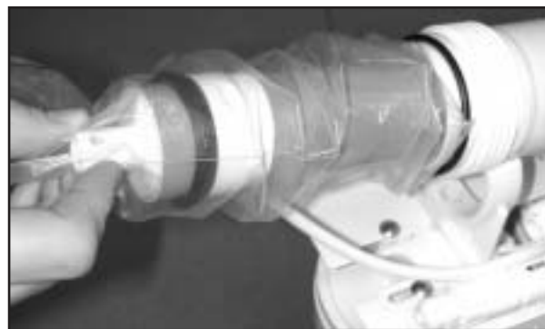
Figure 8 - Installing membrane without touching
