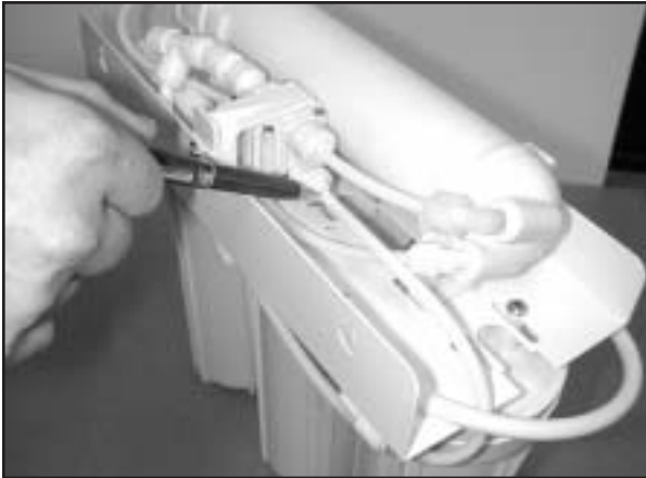
Figure 9 - Disconnect pre-carbon outlet tube from shutoff valve
